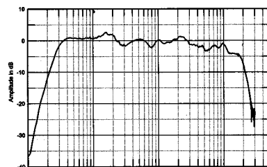
Fig.5 Infinity Epsilon, anechoic response on L-EMIM axis, 37" from floor, at 45" averaged across 30° horizontal window and corrected for microphone response, with complex sum of nearfield woofer and L-EMIM responses below 312Hz.
